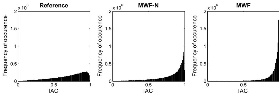
**Fig. 2:** Histograms of the estimated IAC for an example speech stimulus with an input SNR of  $-4$  dB for the reference, MWF-N, and MWF conditions.
