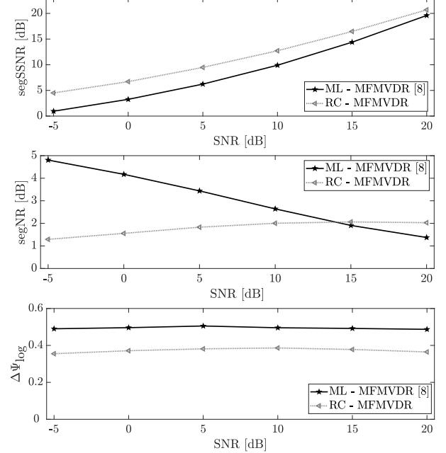
**Fig. 4:** Average segSSNR, segNR and  $\Delta\Psi_{\log}$  using the ML estimate  $\hat{\gamma}_x^{\text{ML}}(m)$  and the RC estimate  $\hat{\gamma}_x^{\text{RC}}(m)$  for different SNRs.
