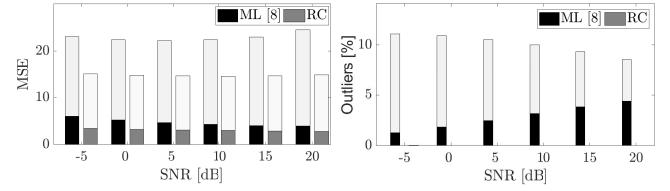
**Fig. 3:** Average MSE and percentage of outliers for the ML and RC speech correlation vectors. The lower and upper parts of the bars represent the performance in speech-and-noise and noise-only, respectively.
